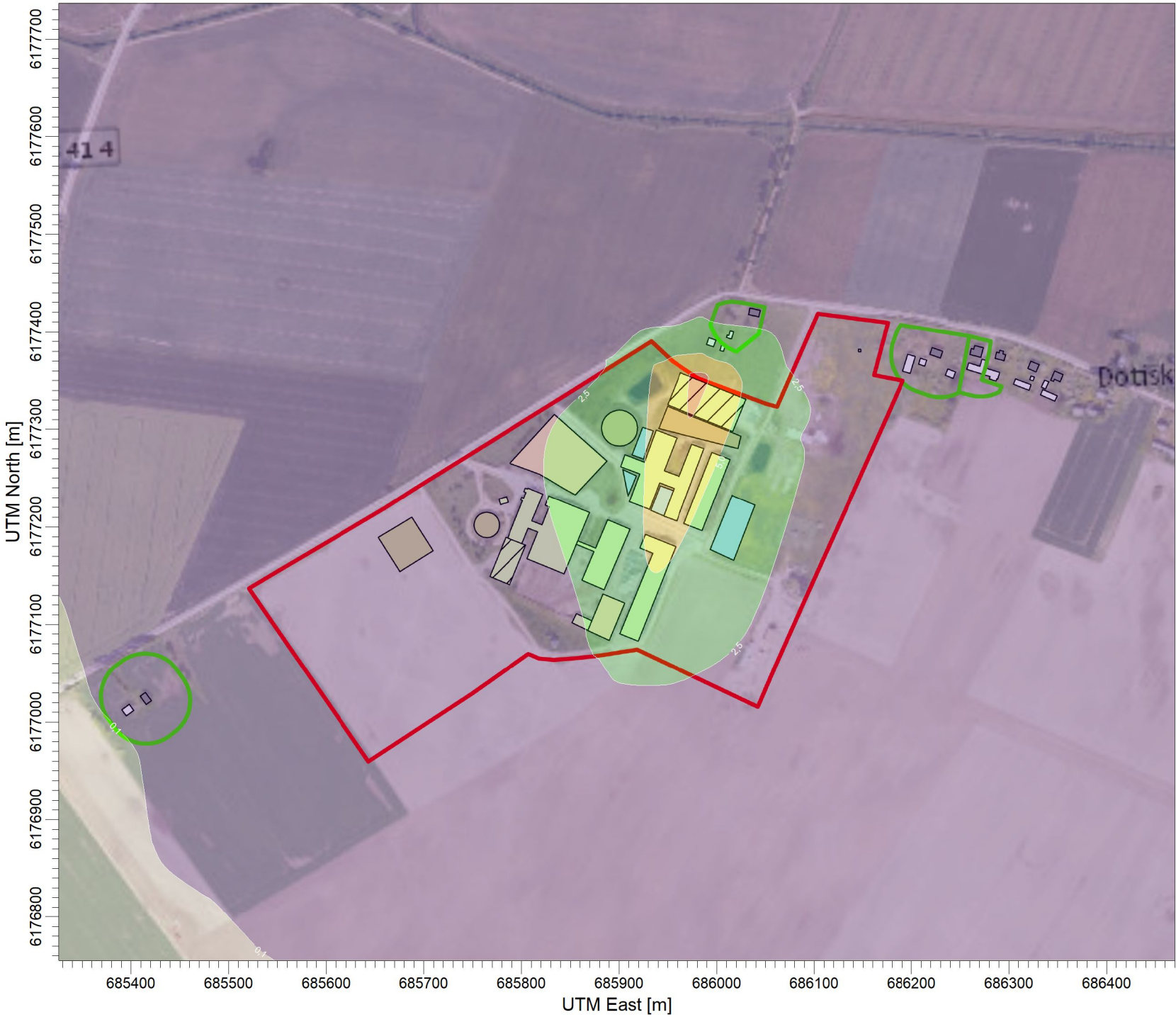
PLOT FILE OF 90.40TH PERCENTILE 24-HR VALUES FOR SOURCE GROUP: PUV Max: 8,2 [ug/m^3] at (685982,15, 6177354,55)
