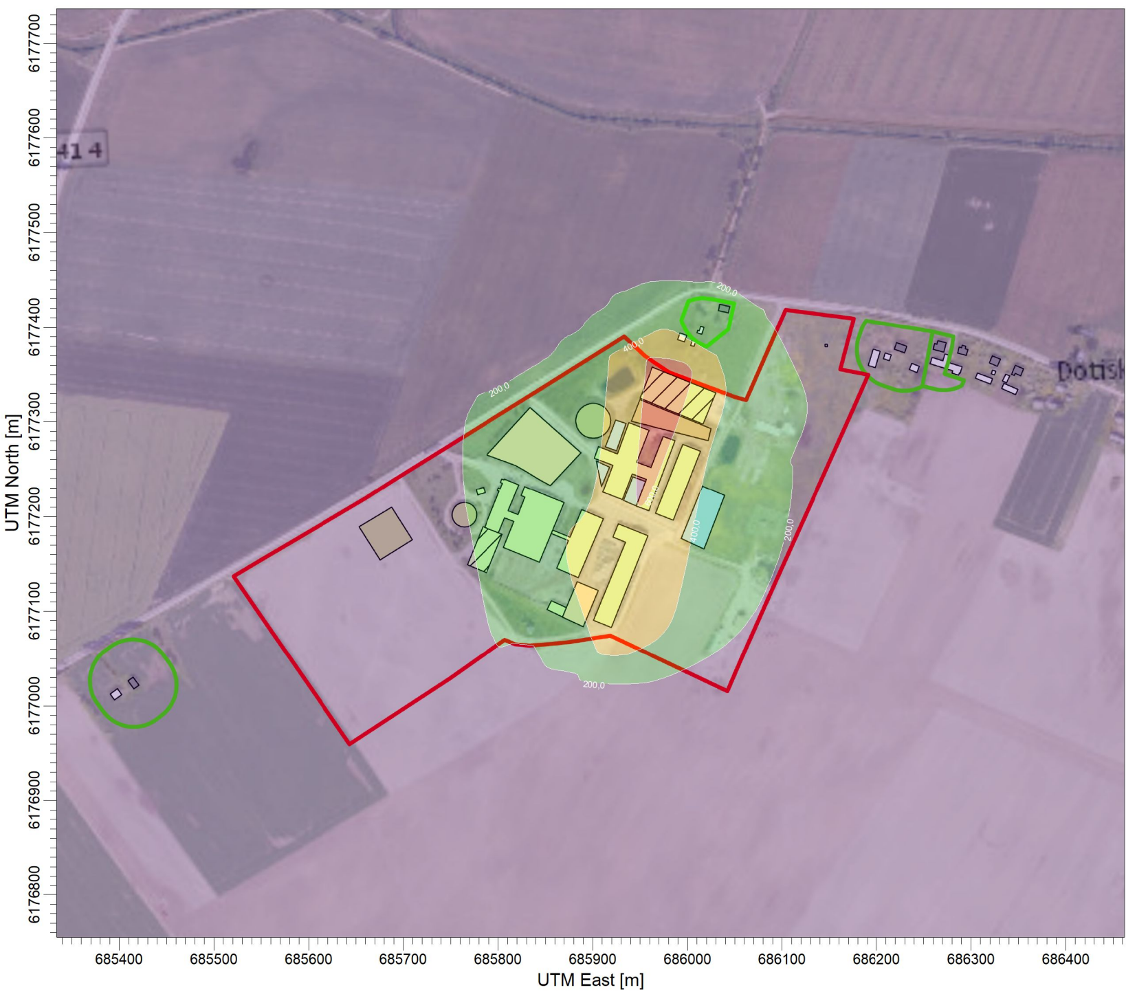
PLOT FILE OF 98.50TH PERCENTILE 1-HR VALUES FOR SOURCE GROUP: PUV Max: 735,1 [ug/m^3] at (685982,15, 6177354,55)
