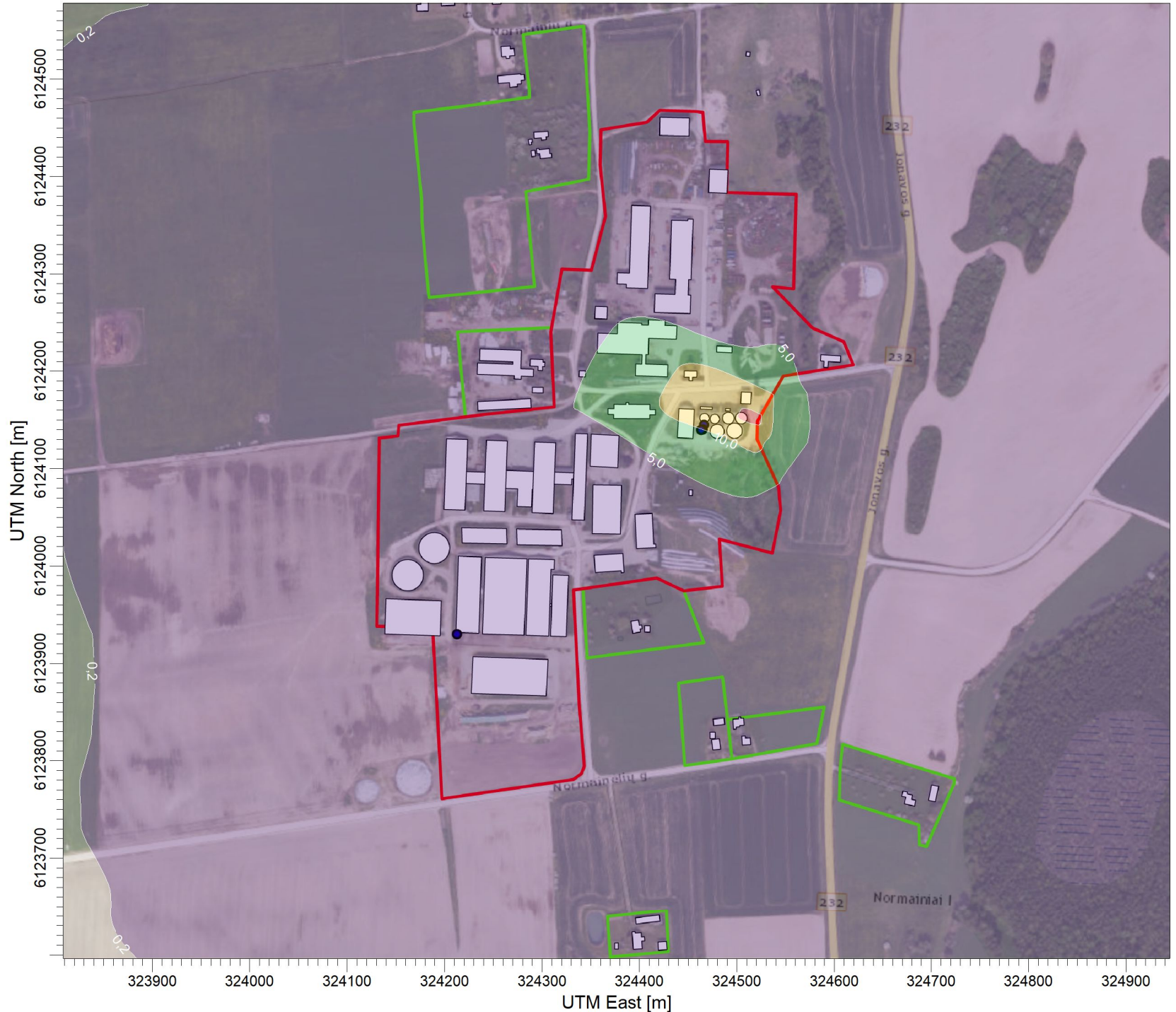
PLOT FILE OF 90.40TH PERCENTILE 24-HR VALUES FOR SOURCE GROUP: PUV Max: 16,3 [ug/m^3] at (324521,84, 6124149,76)
