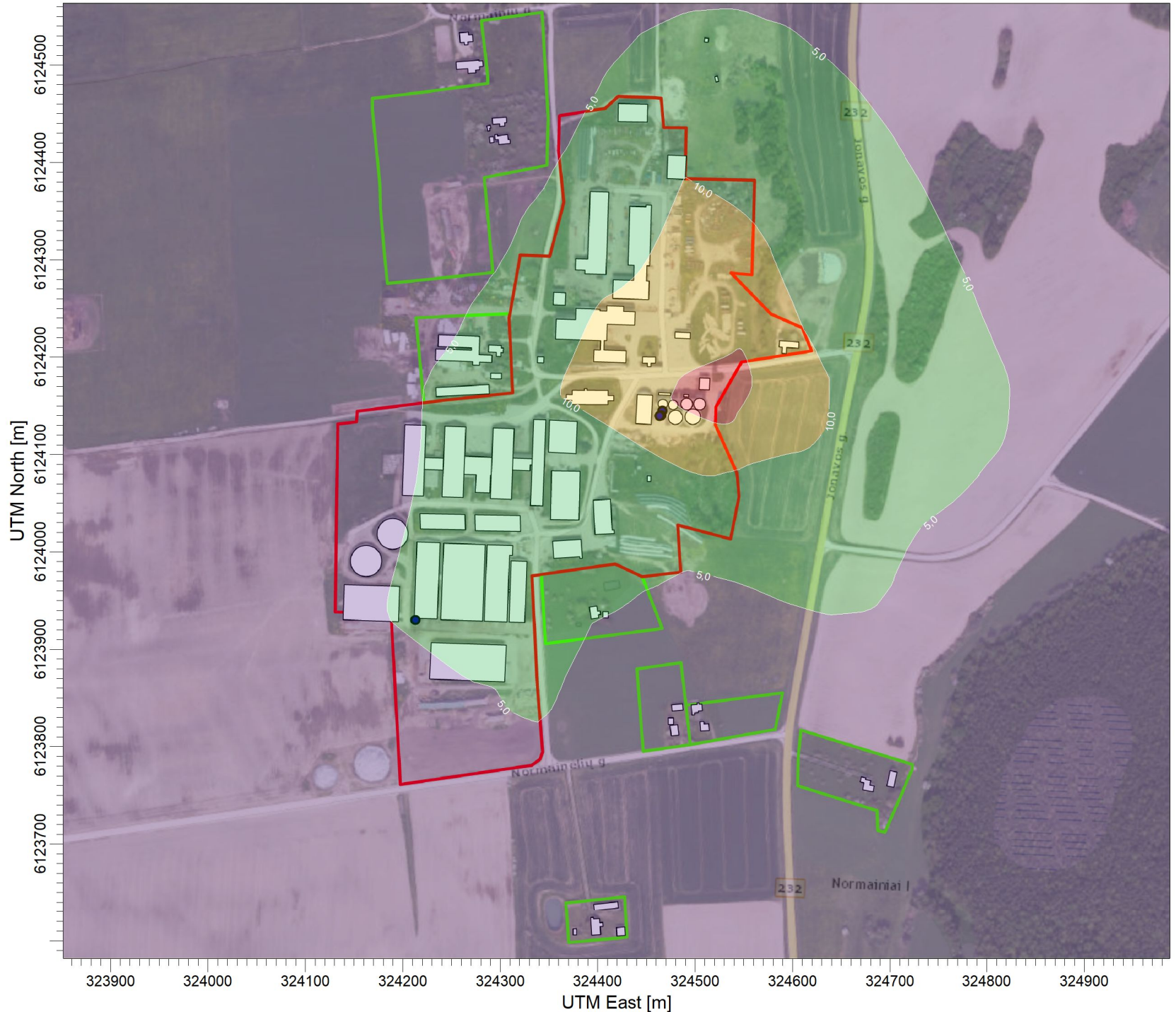
PLOT FILE OF ANNUAL VALUES AVERAGED ACROSS 5 YEARS FOR SOURCE GROUP: PUV Max: 17,1 [ug/m 3 ] at (324521,84, 6124149,76)
