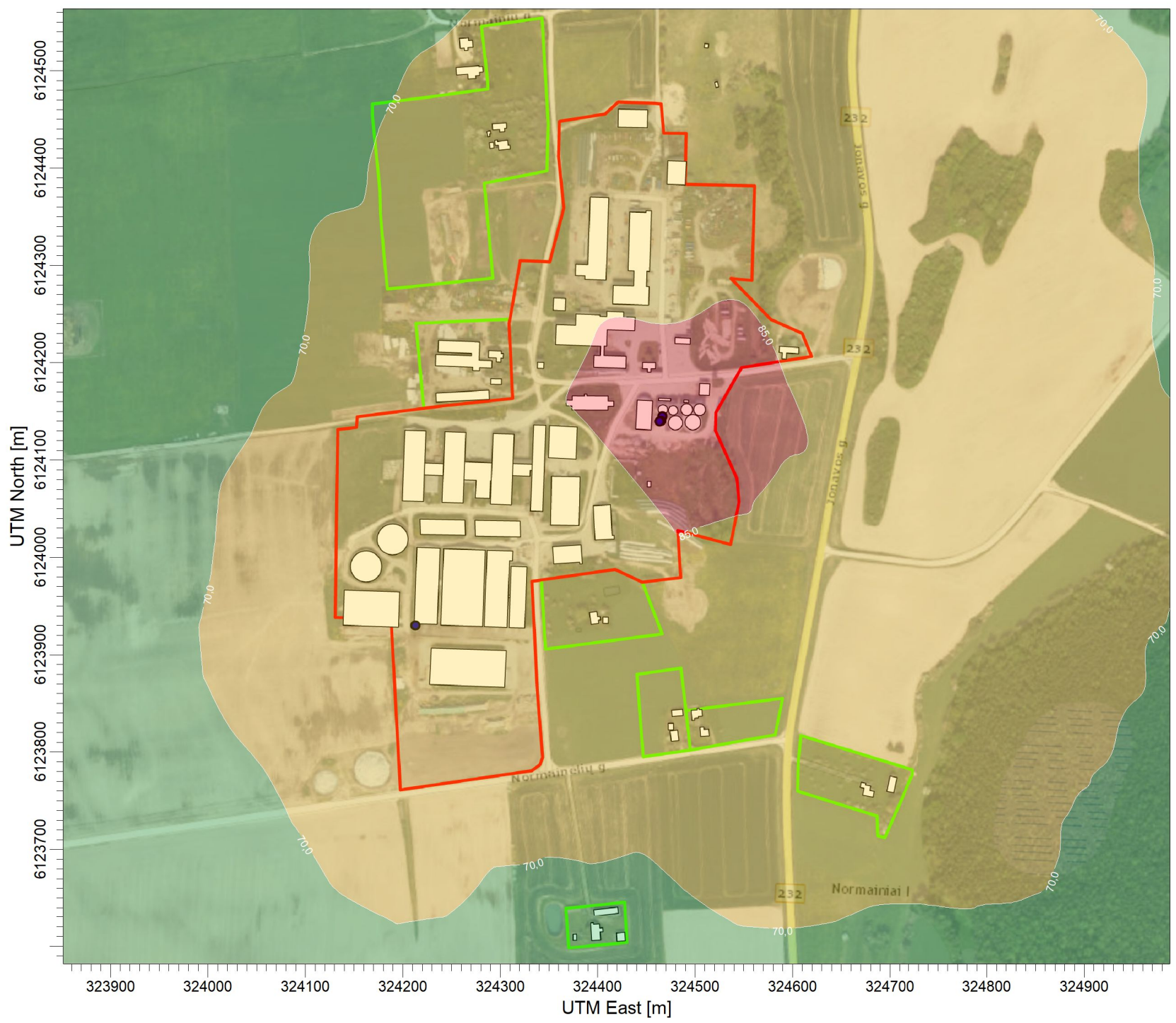
PLOT FILE OF 99.80TH PERCENTILE 1-HR VALUES FOR SOURCE GROUP: ALL Max: 97,7 [ug/m^3] at (324521,84, 6124149,76)
