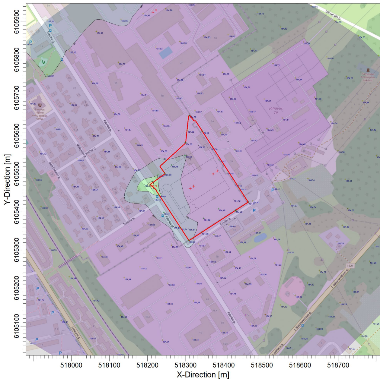
PLOT FILE OF HIGH 1ST HIGH 8-HR VALUES FOR SOURCE GROUP: CO ug/m^3 Max: 187,70 [ug/m^3] at (518207,07, 6105472,05)
