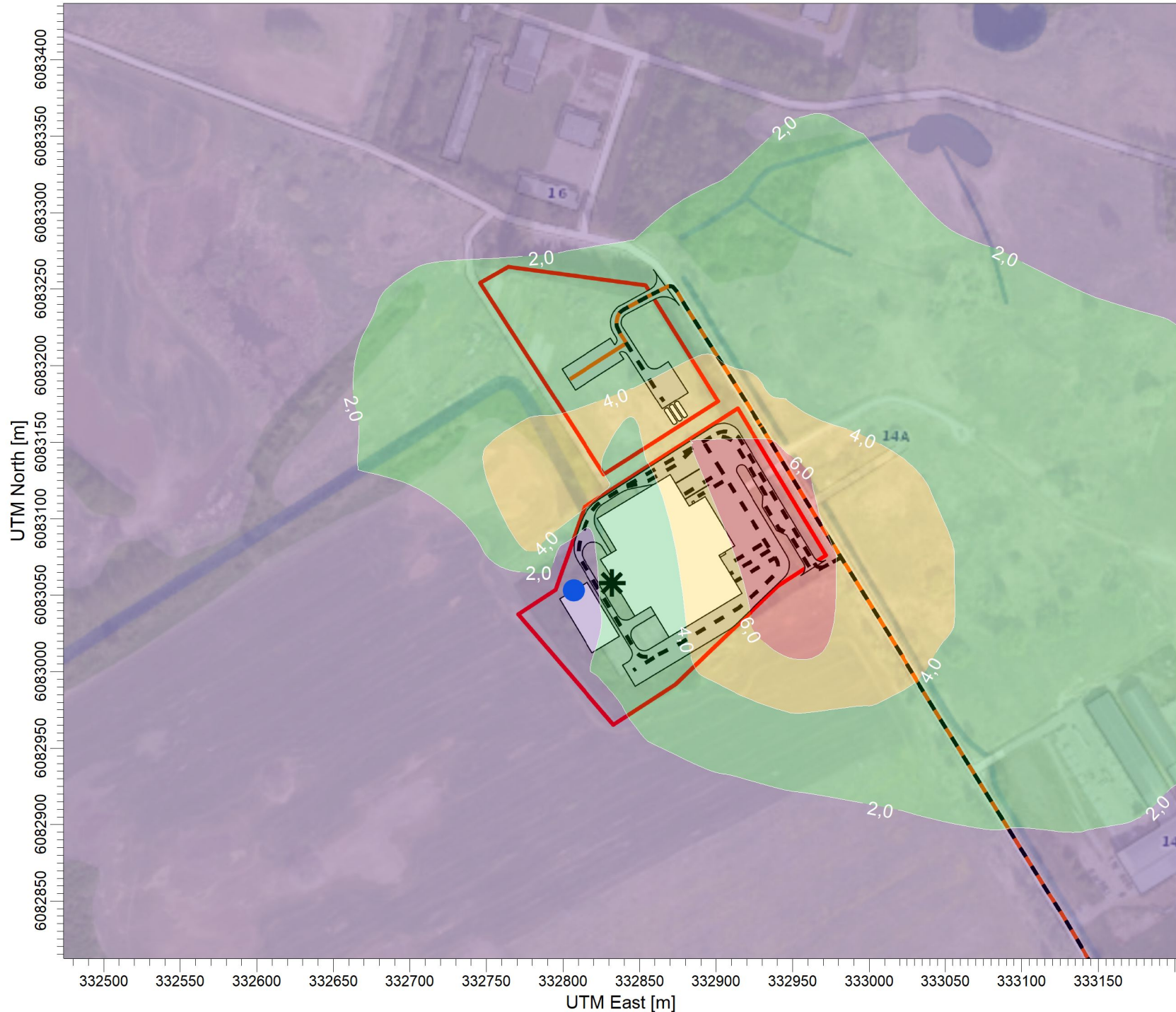
PLOT FILE OF 98.50TH PERCENTILE 1-HR VALUES FOR SOURCE GROUP: PUV Max: 7,6 [ug/m^3] at (332946,29, 6083032,37)
